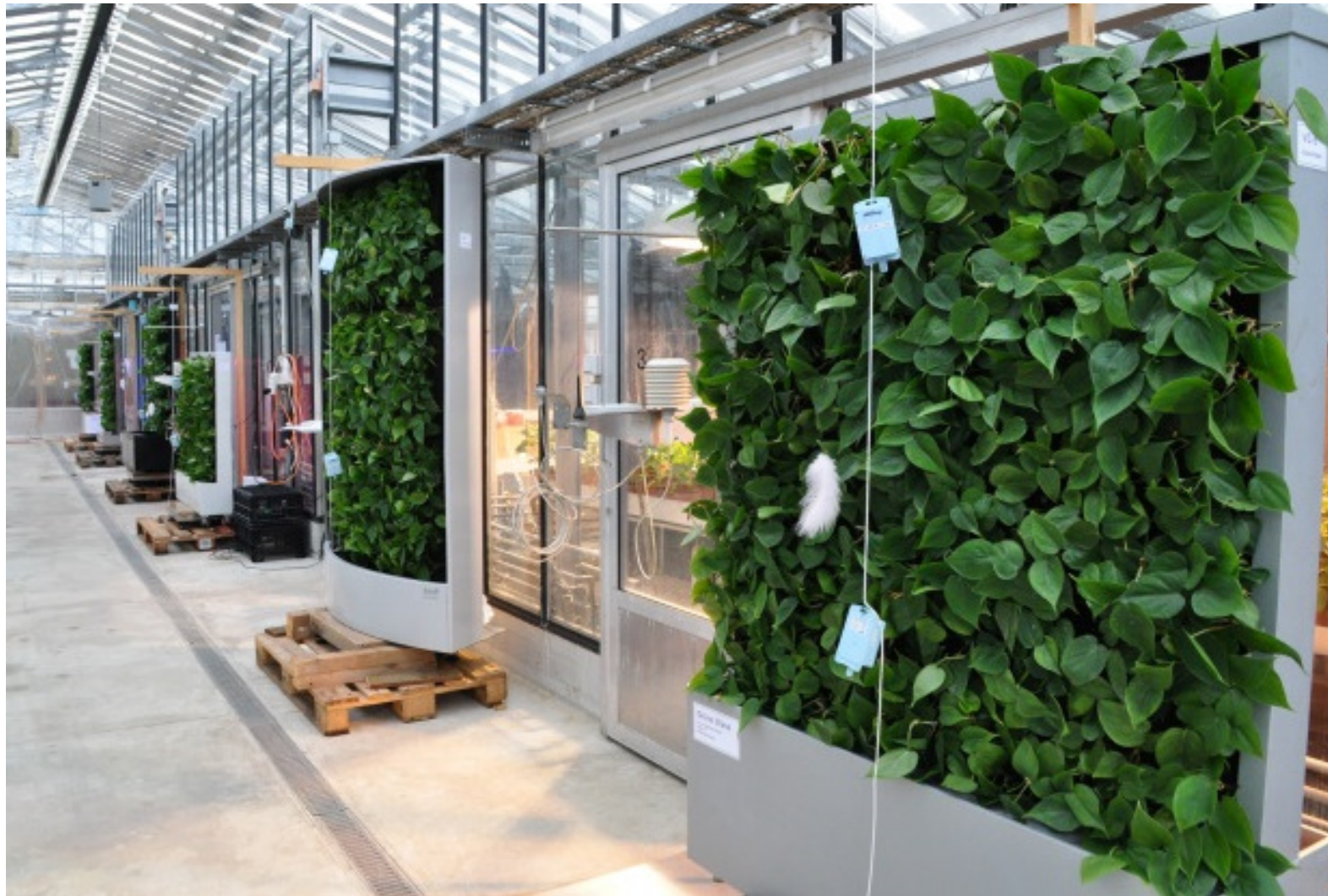
Experimental setup: Vertical greening systems with plants were placed on scales in the greenhouse
